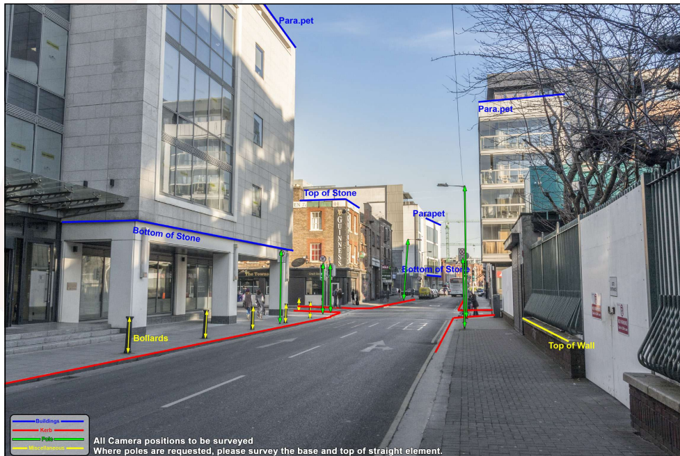
Fig.7: Fixed reference points marked for surveyor in each chosen baseline photo.
