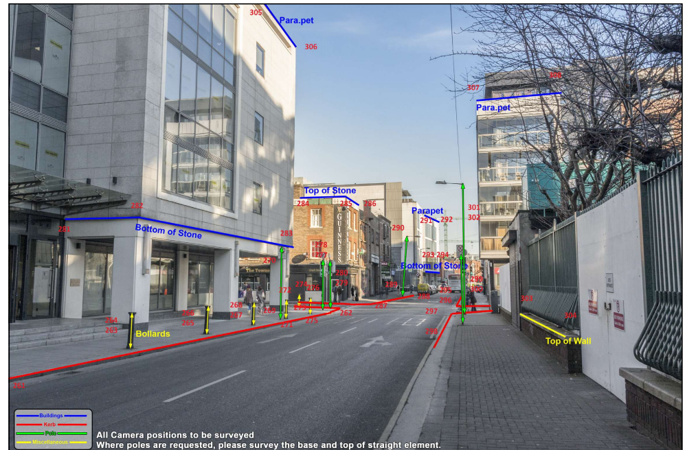
Fig.8: Fixed reference points fully surveyed and numbered.
